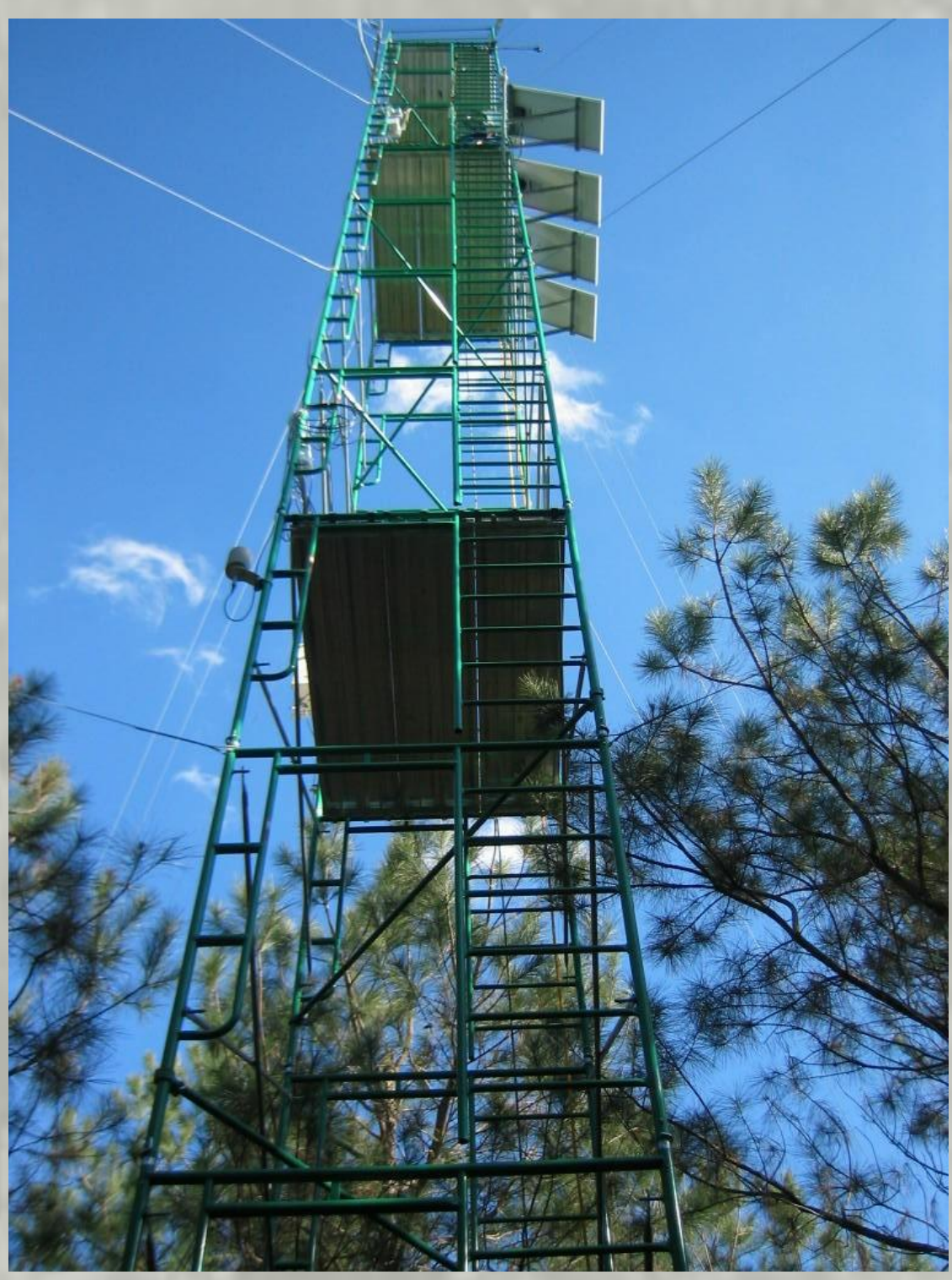
Ameriflux tower in a loblolly pine plantation on the coastal plain of North Carolina
