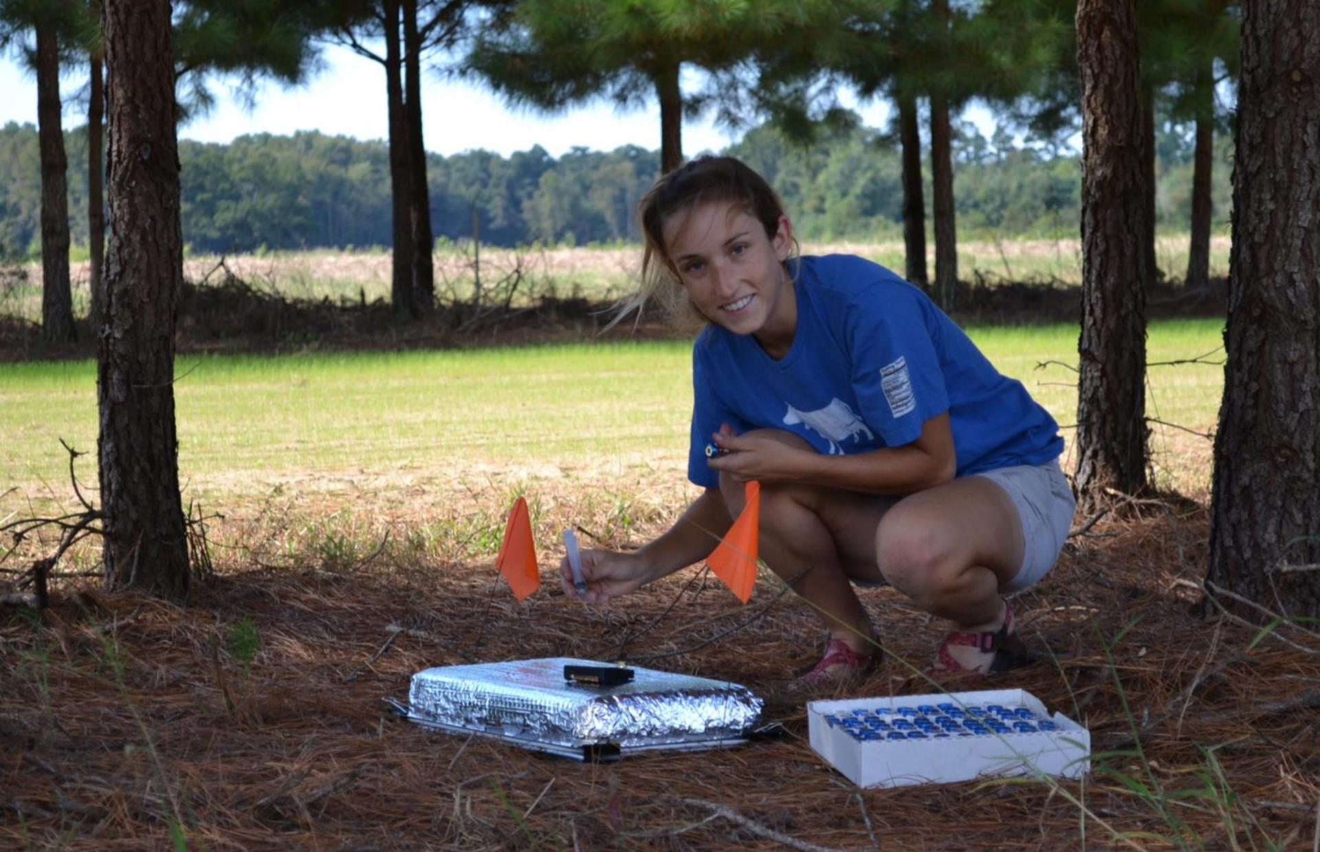
Ms. Janet Chappell (M.S. candidate at NCSU) collecting gas samples for optimizing chamber deployment time and number of locations
