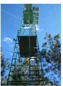
A 70-ft. tower built in 2004 was instrumented to continuously measure carbon and water fluxes in a 15-year-old loblolly pine plantation on the coastal plain of eastern North Carolina. (Photo by Ge Sun)
