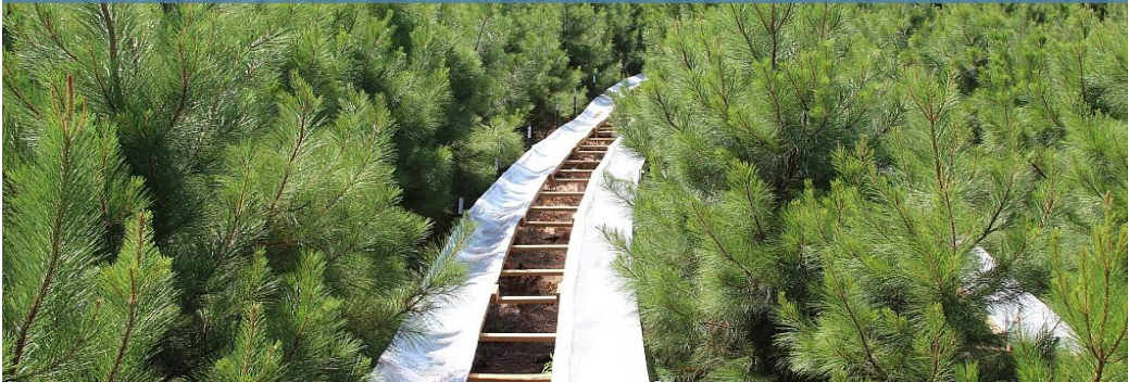
PINEMAP research site diverts rainfall to simulate future precipitation changes (page 2). Photo courtesy of Duncan Wilson.
