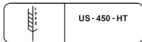
Fig. 6.4 Example of an approved stamp for solid wood packing materials. The stamp, denoting the country of origin, the treatment facility, and the treatment type, signifies that a piece of wood has been treated in compliance with International Standards for Phytosanitary Management (ISPM 15) from the International Plant Protection Convention
