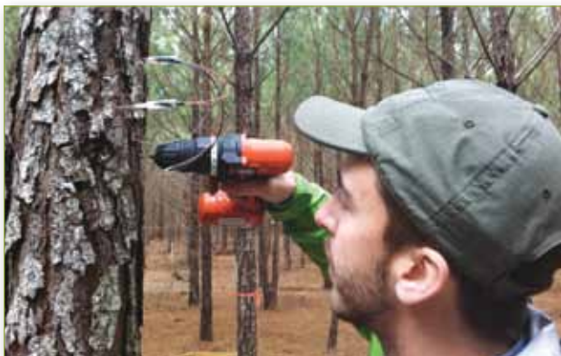
Figure 6.1. University of Florida M.S. student Maxwell Wightman drills a hole to insert thermal dissipation sensor probes into a tree at the Tier III site in Florida. Photo by Geoffrey Lokuta.
