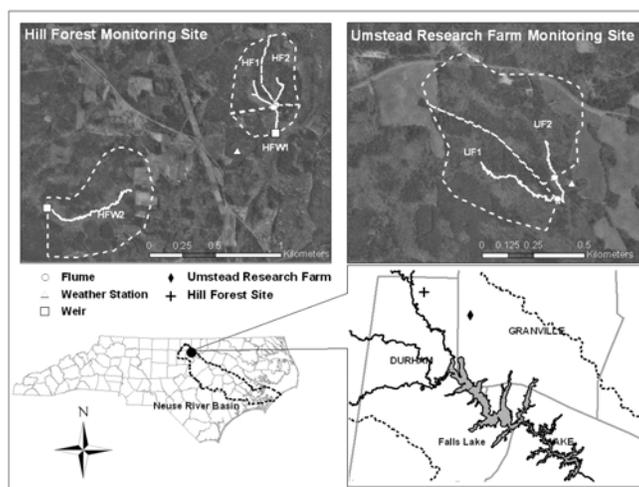
Figure 1. Watershed, weir, flume, meteorological station and stream temperature monitoring locations. Continuous stream temperature monitoring locations are at the flumes and weirs.
